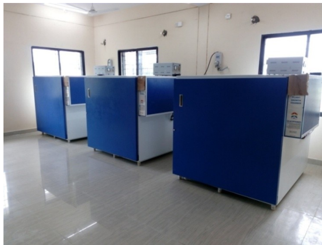
Environmental /Plant Growth Chambers with CO 2 , Temperature, Relative Humidity and Light regulation
