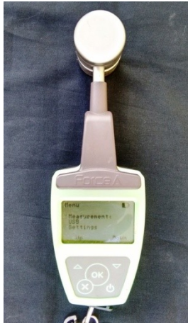
Dualox Scientific sensor used for Leaf chlorophyll, flavonoids, Nitrogen balance index and anthocyanin measurement
