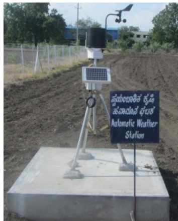
Automatic Weather stations
